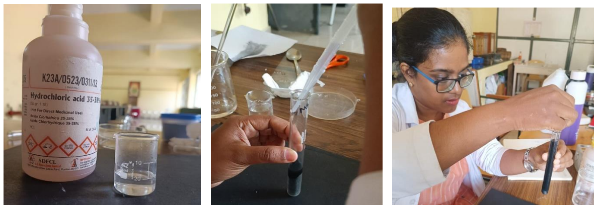
Fig. 26: Preparation of solution of sample with 20% Hcl
