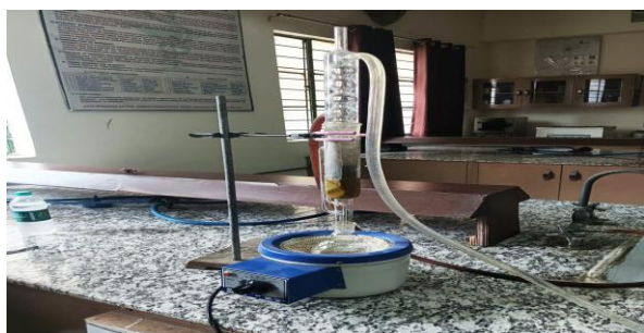
Figure: 2 Soxhlet extraction process
