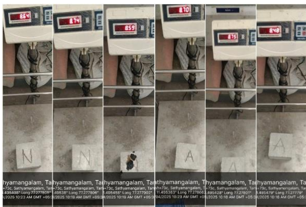
Figure 4. Water absorption test
