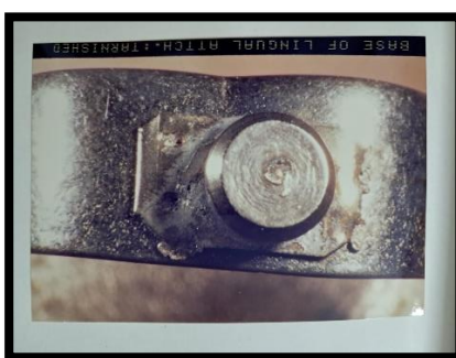
Fig 3: Surface corrosion around the lingual button on the band.
