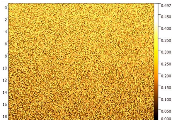
Picture 1: Microscopic images captured using Atomic Force Microscopy showcases reciprocating files before they undergo instrumentation, with the image representing a scale of 10 micrometers by 10 micrometers. The images feature: ProTaper Gold, recognized for its innovative design. This file intricate details are highlighted at the microscopic level ( \mu\text{m} =micrometers)
