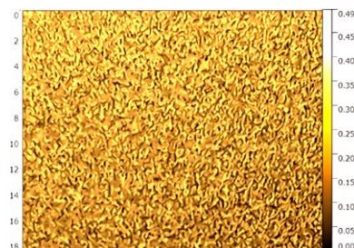
Picture 2: Microscopic images captured using Atomic Force Microscopy showcases reciprocating files before they undergo instrumentation, with the image representing a scale of 10 micrometers by 10 micrometers. The images feature: WaveOne Gold (WOG), known for its efficiency. This files intricate details are highlighted at the microscopic level ( \mu\text{m} =micrometers)
