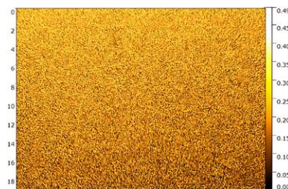
Picture 3: Microscopic images captured using Atomic Force Microscopy showcases reciprocating files before they undergo instrumentation, with the image representing a scale of 10 micrometers by 10 micrometers. The images feature: EdgeOne Fire (EOF), which is engineered for optimal performance in endodontic procedures. This files intricate details are highlighted at the microscopic level ( \mu\text{m} =micrometers)
