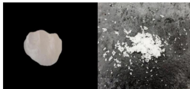
Figure 2: The light cured nanoparticle incorporated composite block and its powdered form (from left to right)
