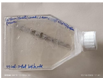
Figure 2: Formation of biofilm on the stainless-steel implant.
