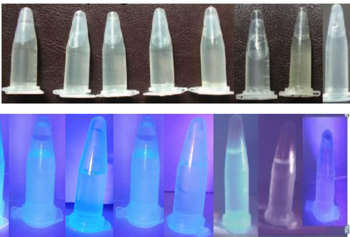
Fig 06: CDs, CDs+ \text{Pb}^{2+} , CDs+ \text{Cu}^{2+} , CDs+ \text{Cr}^{3+} , CDs+ \text{Ni}^{2+} , CDs+ \text{Co}^{2+} , CDs+ \text{Fe}^{+3} , CDs+ \text{Mn}^{7+}
