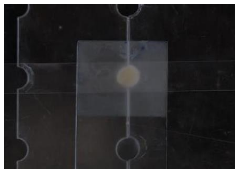
Figure 3 – A glass strip placed over the mold to ensure the removal of the excess
