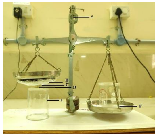
Figure 1: Measurement of mucoadhesion strength using modified physical balance
