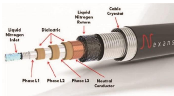
Fig. 4: HTS power transmission cable developed by Nexans SuperConductors GmbH. The concentric arrangement of three phases L1, L2, and L3 allows a very compact cable design. The conducting parts of the cable (L1, L2, L3) consists of a HTS material.
