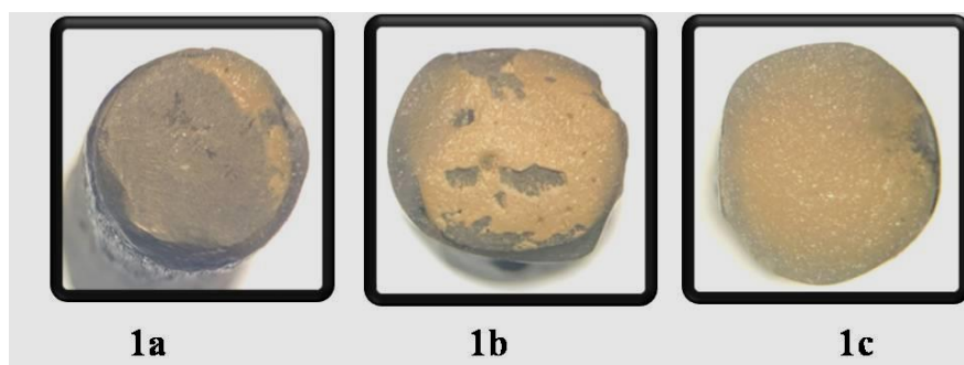
Figure I: Stereomicroscope images at 80x magnifications revealing different types fractures 1a Adhesive fracture between metal ceramic, 1b Mixed type of fracture between metal ceramic and 1d showing Cohesive type fracture
