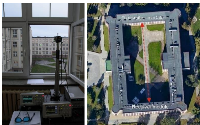
Figure 11. Outside the Military University of Technology building, the laboratory is used to test the FSO link.
