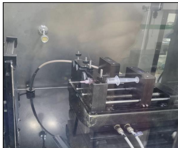
Figure-1A - Electrospinning process of cranberry loaded nanofiber membrane
