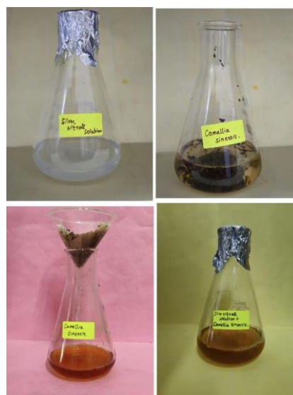
Figure 2: Depicts the preparation of green tea-Silver nanoparticles along with addition of hyaluronic acid and Poly vinyl Alcohol
