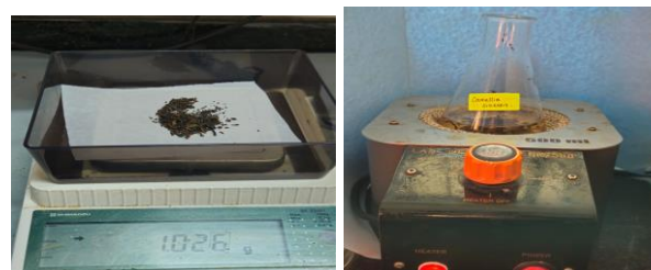
Figure 1: Depicts the weighting of green tea powder and placement in the orbital shaker
