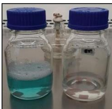
Figure 5: Immersing plates in fittydent solution and distilled water
