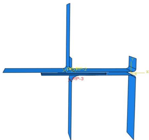
Fig.1: The 3D model in L-die bending of SPCC double-layer sheets
