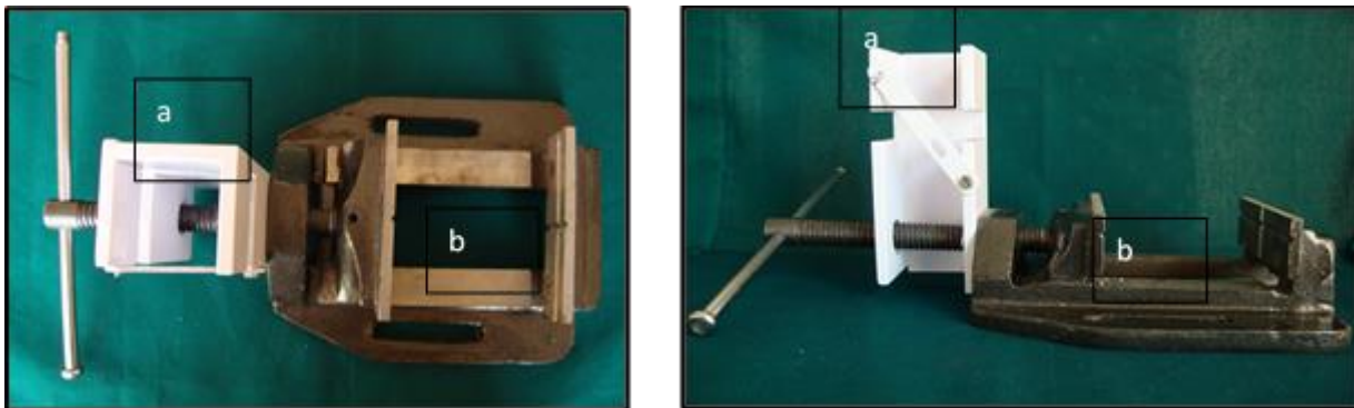
Fig 1: Customized instrument. A- top view. B- Front view a. for stabilizing and moving vernier calliper b. for stabilizing the dental cast.
