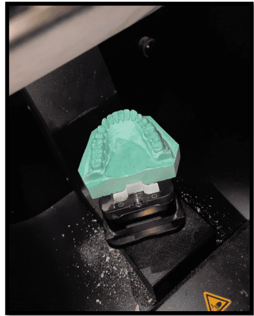
Figure3:Scanningconventionalcastswithdesktop scanner(Ceramill map 400)
