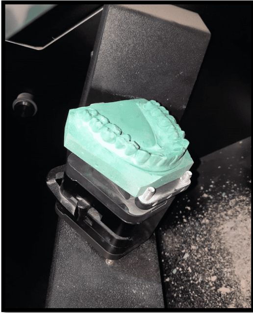
Figure3:Scanningconventionalcastswithdesktop scanner(Ceramill map 400)
