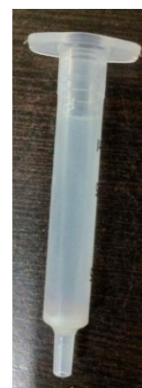
Fig 1: Image of Sephadex Column used for filtration of Emulsomes.
