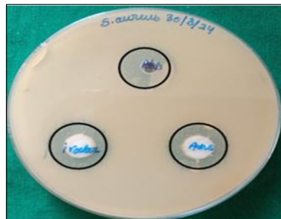
Figure 4 Zone of inhibition for PMMA and bis-acrylate composite resin on staphylococcus aureus
