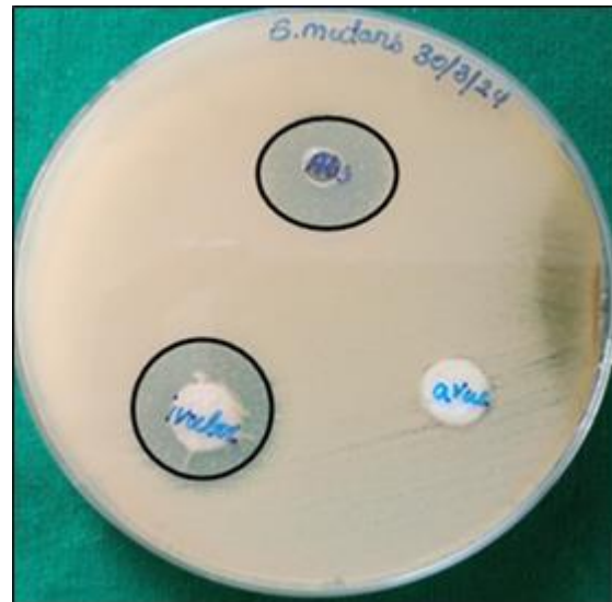
Figure 3 Zone of inhibition assessed for PMMA and bis-acrylate composite resin on Streptococcus mutans
