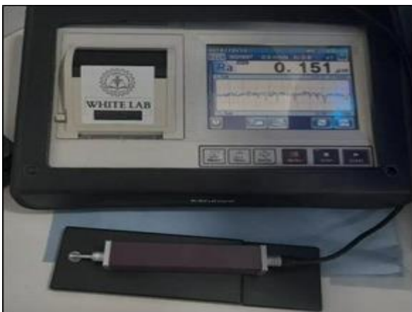
Figure 3 Surface profilometer with the sample
