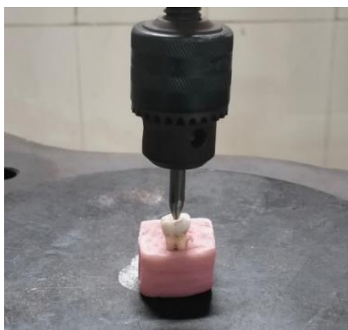
Fig. 4 Compressive loading on Occlusal Surface of Molars in Universal Testing Machine
