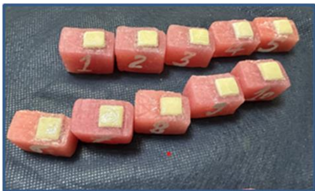
Figure (1) The intact ceramic-metal samples after being cast in acrylic bases, trimmed, and numbered .
