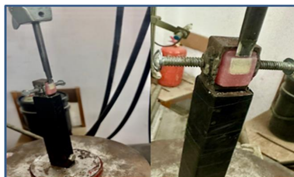
Figure (5): Application of Shear Force Parallel to the Interface Surface.
