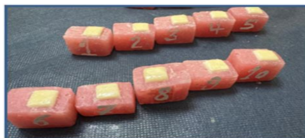
Figure (2) The intact zirconia ceramic samples after being cast in acrylic bases, trimmed, and numbered .
