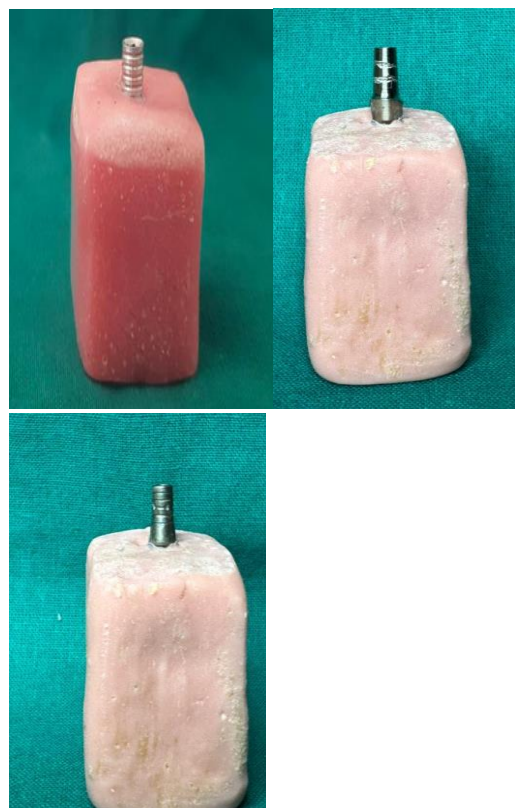
Abutment mounted in lab analog and surface modification techniques applied.
