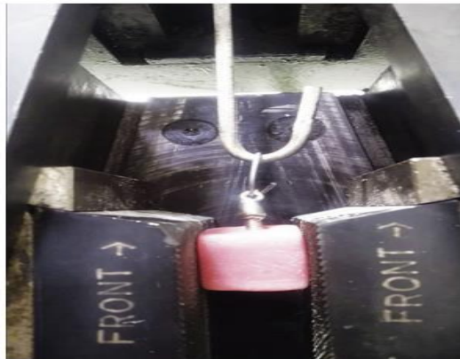
Figure 4. Universal testing machine performing tensile test.
