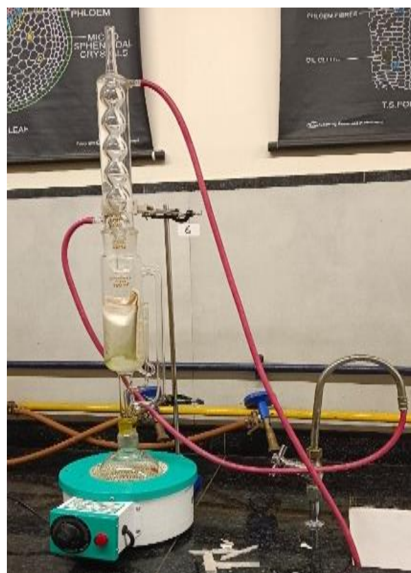
Figure 1. Soxhlet extraction apparatus
