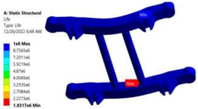
Figure 19. Fatigue life cycles from the simulation at 60 mm wheel flat length
