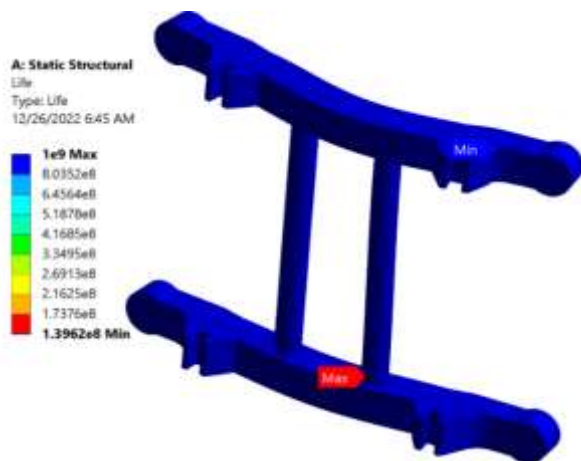
Figure 18. Fatigue life cycles from the simulation at 40 mm wheel flat length
