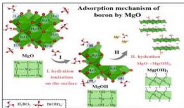
Figure 4: Schematic diagram of boron adsorption and hydration of MgO [75].
