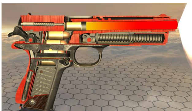
FIGURE 2 Screen capture from the WoG mid-discharge of the Colt Model 1911 in cutaway mode. Observable is the gas pressure, shown as a color gradient, behind the projectile which has just been expelled from the muzzle.
