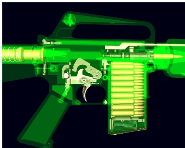
FIGURE 3 Screen capture from the WoG of the Colt M16 A1 in one of the x-ray modes where some parts are still visible. Observable are the trigger mechanism, gas tubes for the direct impingement into the bolt carrier group, and the cartridges in the magazine and chamber.
