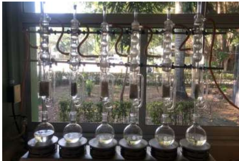
Photograph 9. Determination of fats and oils by the reflux method with Soxhlet equipment
