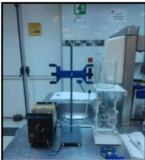
Figure 2. Illustration of the assembly to establish the breakout curve.
