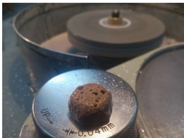
Figure 2: Image of the disc grinder and produced glass foam.
