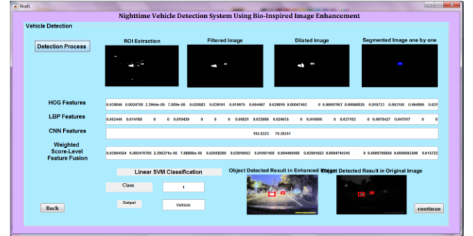
Figure 5. ROI, Feature Extraction, SVM classification, Detection Results
