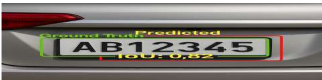
Figure 9: YOLOv5 License Plate Detection – Bounding Box and IoU Demonstration
