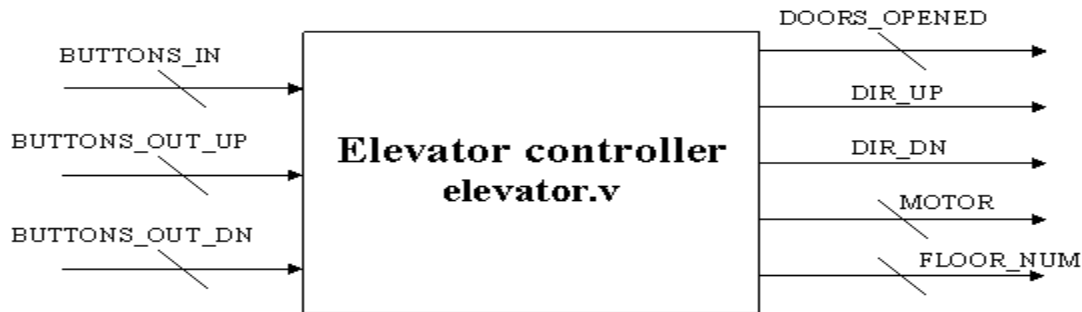
Fig :1. Lift control system
