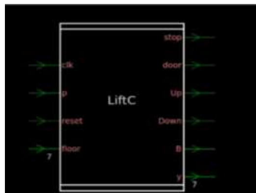
Fig:2. Pin diagram of lift
