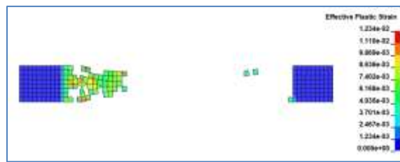
Fig. 8. Fracture in the tensile simulation of the chitin-graphene specimen
