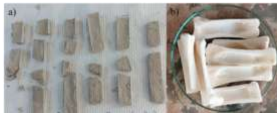
Fig. 1. a) Chitin/graphene samples. b) Bone samples
