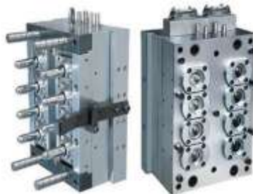
Figure 1: Injection mould used for making multiple bottle caps
