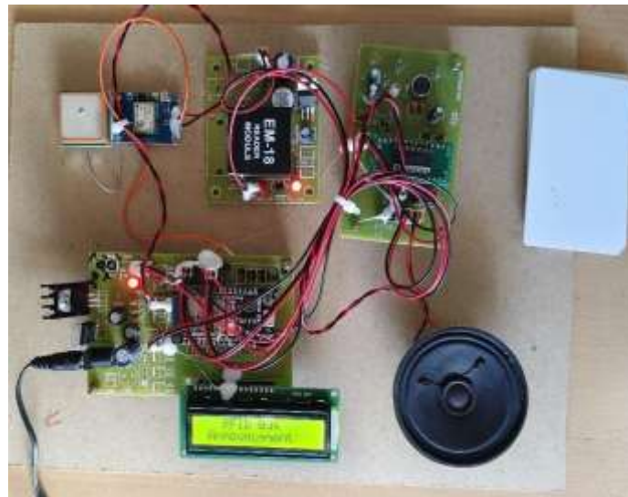
Fig. 5: This image shows an RFID-based bus announcement system in the 16x2 LCD display.
