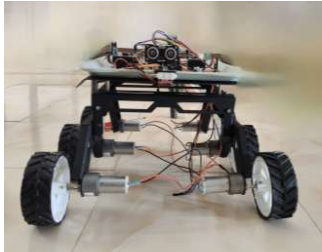
Fig. 3: Six-wheeled robot with a Rocker-bogie suspension system
