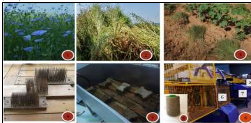
Figure 1: 1) Flax Plant 2) Collection of plants 3) Drying process 4) Rippling process 5) Water retting 6,7) Setup for breaking and scutching of fibres from stalk. 8) Flax fibre rolls 9) Final produced Fabric
