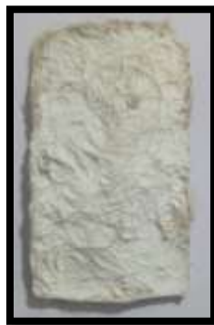
Fig. 2 Stable specimen obtained with 44.4% w/w fiber-resin ratio
