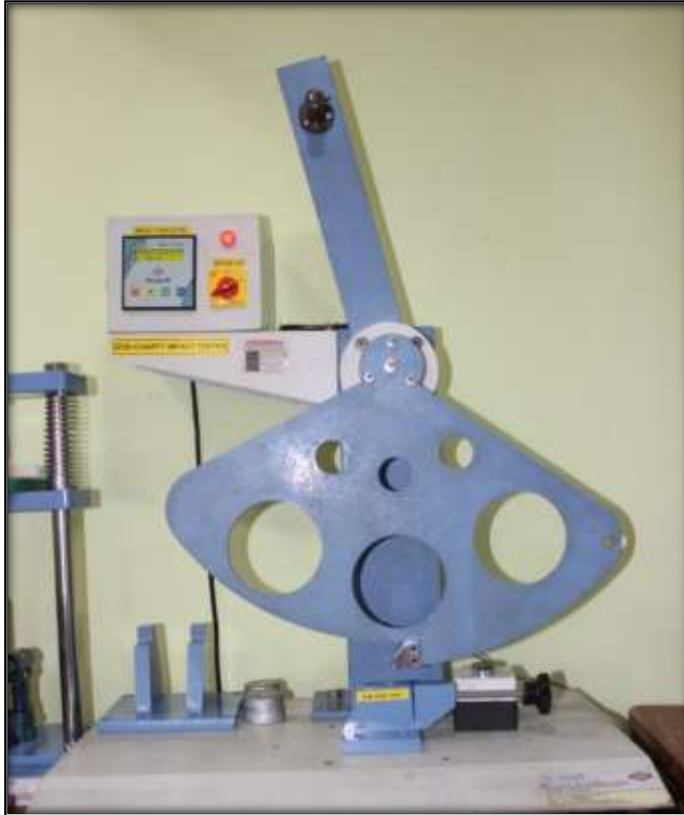
Fig 4. Visualization of the specimen loaded for Impact test
