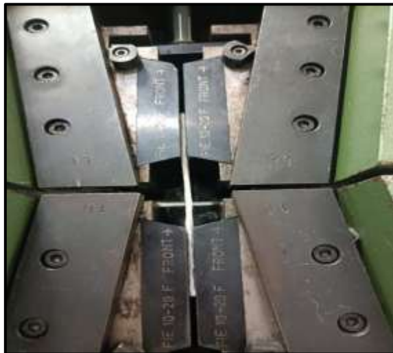
Fig 2. Visualization of the specimen loaded for tensile test
