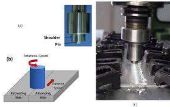
Figure 1. (a) A simple FSW tool, (b) a schematic of the FSW process, and (c) a setup of FSW illustrating the specially designed fixture.
