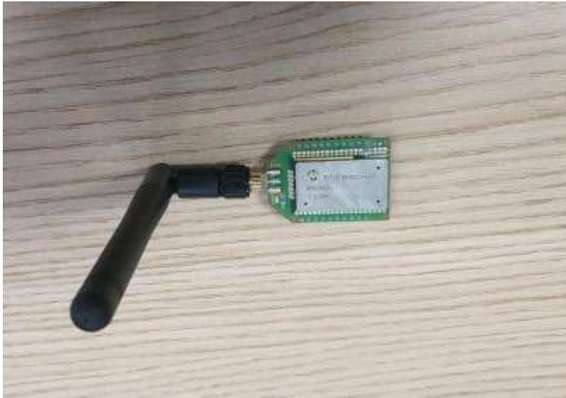
Figure 2.2: RN2483LoRaWAN communication module
