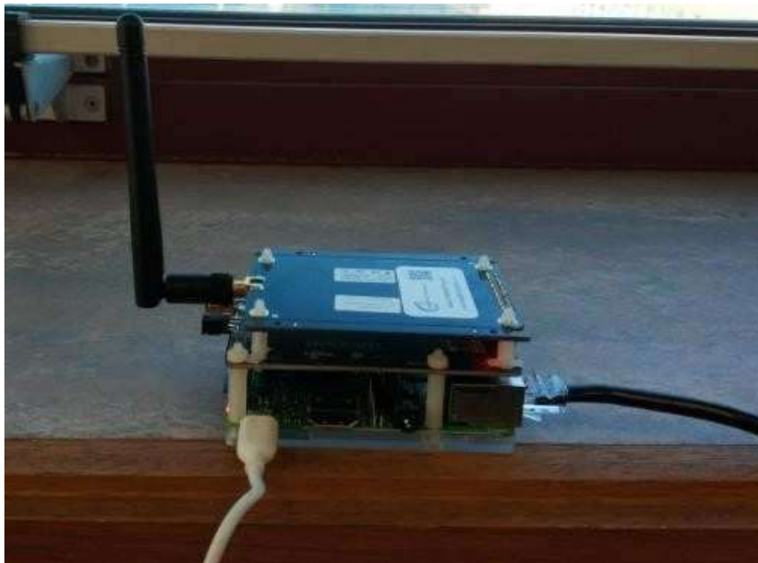
Figure 2.5: The LoRaWAN gateway
