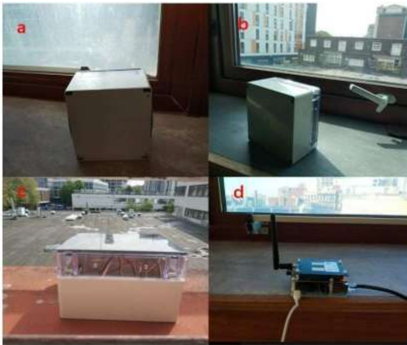
Figure 3.1: The deployment of sensor nodes and the LoRaWAN gateway. (a) Sensor node in indoor condition; (b) Sensor node in indoor condition (alternative angle); (c) Sensor nodes in outdoor condition; (d) LoRaWAN gateway in indoor condition.
