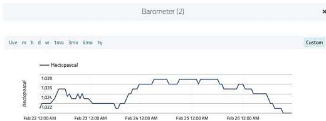
Figure 3.3: The measured air pressure over 5 days
