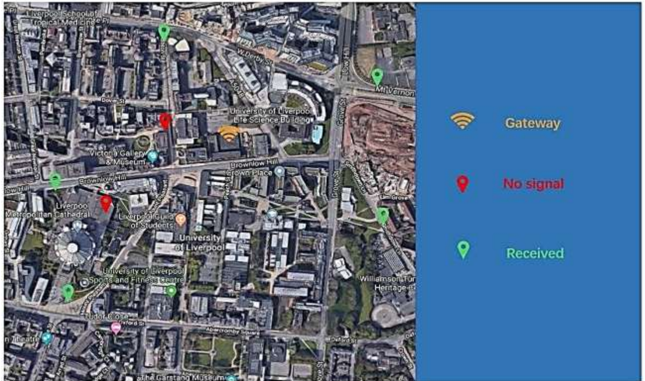
Figure 3.8: LoRaWAN's test of coverage
