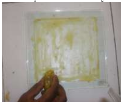
Fig: 2.3 applying Wax to the mould
