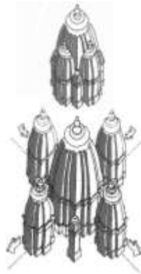
Fig. 15 Conceptually embedded aedicules in a Nagara temple. Source: Adam Hardy, Indian Temple Typologies
