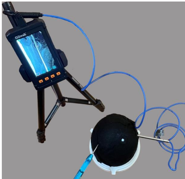
Figure 3: Complete L-CASST simulator
