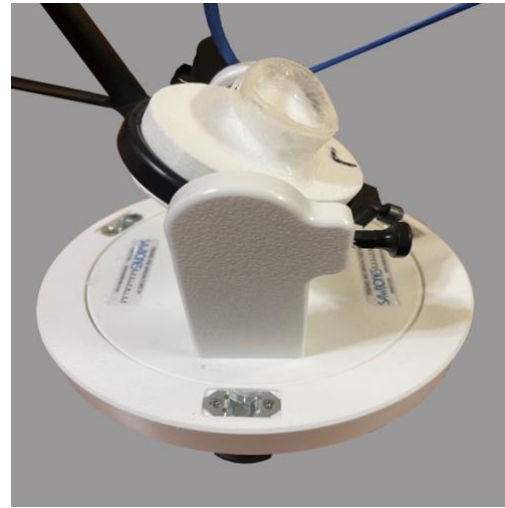
Figure 2: Glenoid base used for the L-CASST simulator
