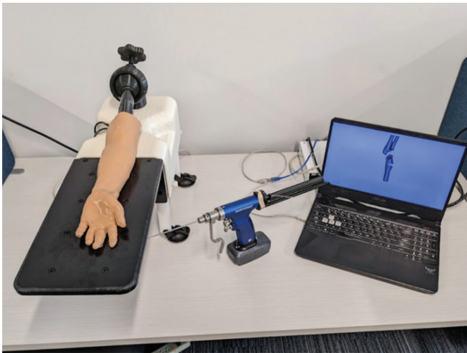
Figure 4. Pediatric supracondylar humeral fracture simulator with 3D printed bony anatomy, real-feel fracture reduction capabilities, true surgical instrumentation compatibility, and real-time radiation-free “fluoro” imaging available.
