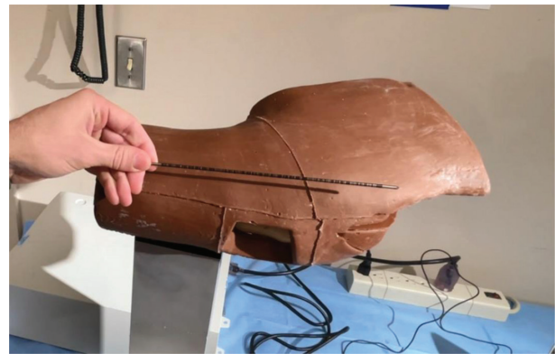
Figure 2. Laser-etched bar-coding on guidewire allows cameras to determine the exact position and orientation of the wire in space. The wire location is correlated with the position of the sawbones model within the soft tissue envelope and allows for the simulation model to project a “fluoro” image on the computer screen at any point during the exercise.
