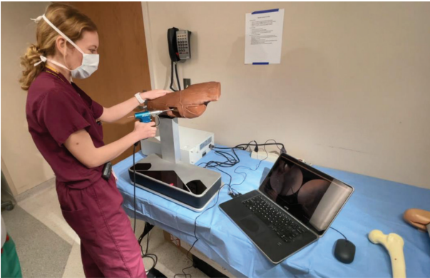
Figure 3. Photo image of an orthopaedic resident working through the simulation model tasks. Participants have a foot pedal (not pictured) that allows them to obtain AP and lateral “fluoro” images at any point during the exercise.
