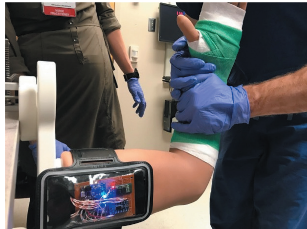
Figure 5. Distal radius fracture model arm and exterior processing and computing hardware in use during a trial reduction and casting experiment.
