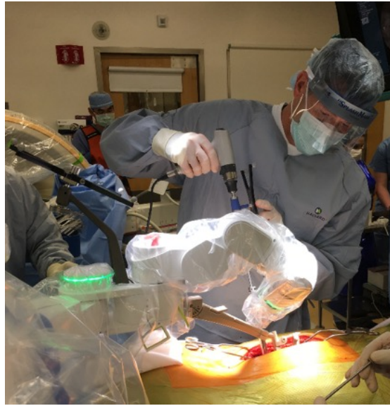
Figure 12. Intraoperative photo of drilling through the robotic arm with navigated instruments.
