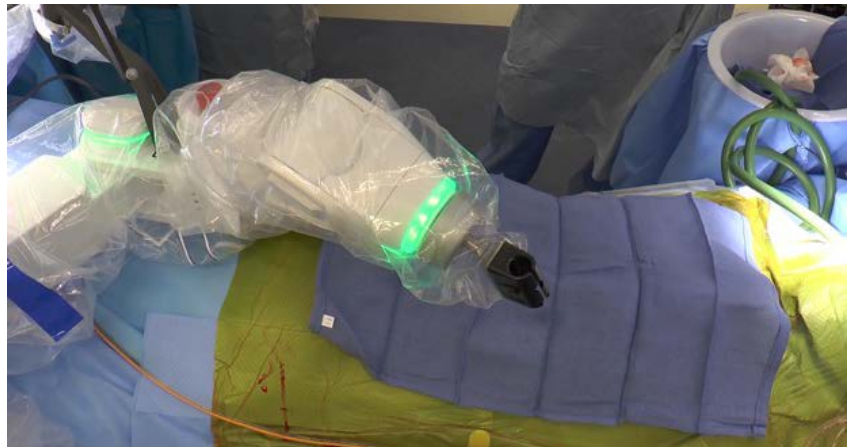
Figure 8. Intraoperative photo of the robotic arm performing an optical scan of the operative field to aid in collision avoidance and efficiency of arm movement.
